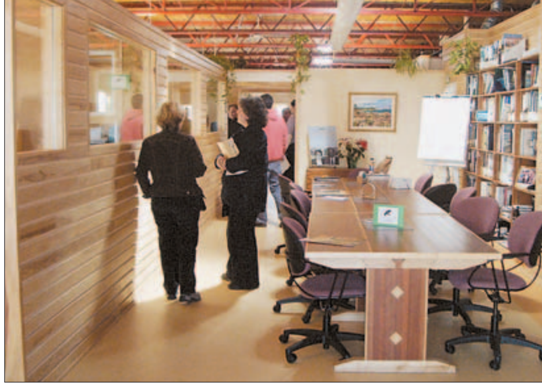
The Michigan Land Use Institute in downtown Beulah was once a house and used many recycled components in its renovation. The conference table is refurbished redwood, once a deck, and the cubicle windows are patio doors turned on their sides.
